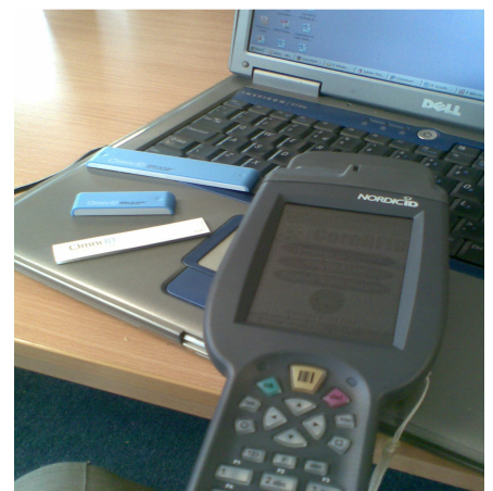
An IT auditor with an RFID equipped PDA can check assets quickly and accurately.
