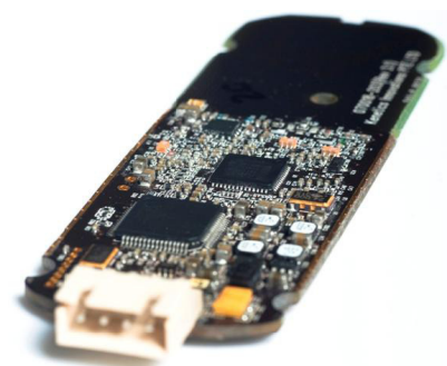
OEM style UHF reader/antenna module with TTL interface for product integration.
