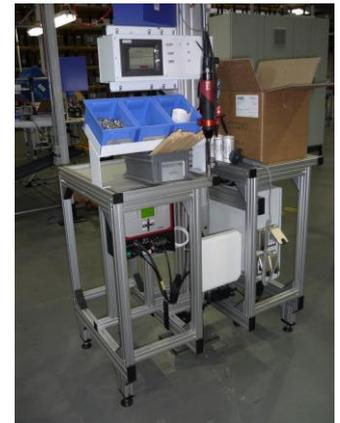
Vaillant Group boiler manufacturing station. The white square in the centre is the RFID reader antenna.
