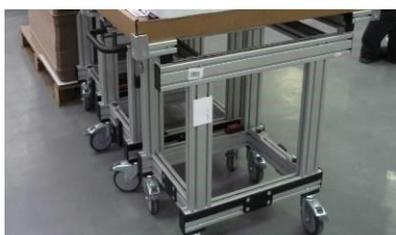
Battery assisted passive RFID tag on a boiler assembly trolley.
