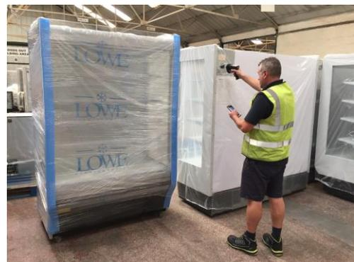
*RFID tags on Lowe's rental equipment allow items to be quickly identified on dispatch, receipt or in the warehouse.*
