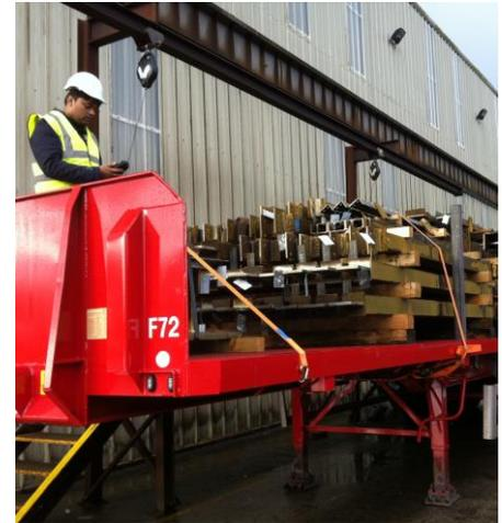
Handheld test reading of RFID tags on steel components on vehicle trolley
