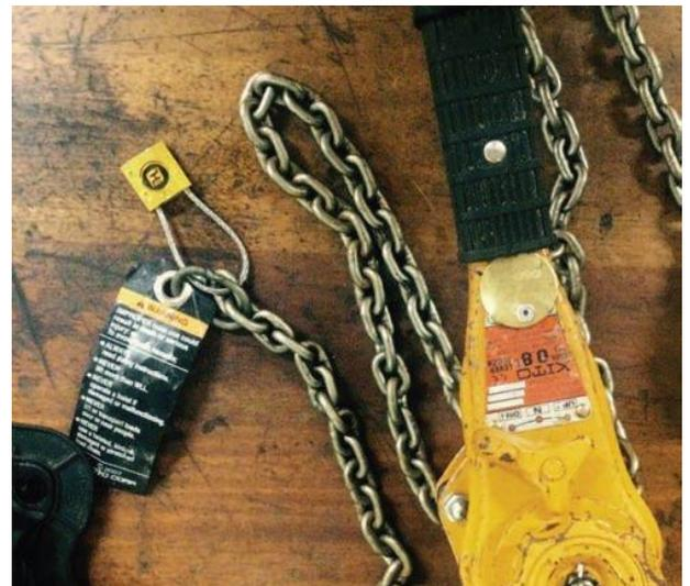
*RFID tags can be easily read to uniquely identify equipment such as tools, tackle and heavy lifting equipment; it's just a matter of picking the right tag for the job.*
