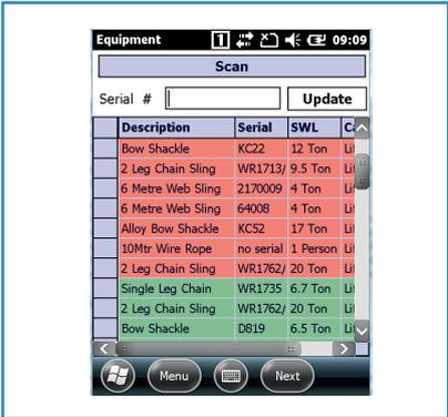
A PDA quickly identifies safe (green) and unsafe (red) items of equipment by scanning tags.
